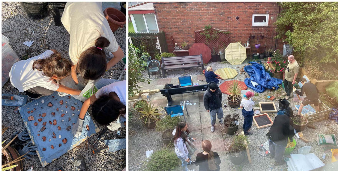
Fig. 9. Ivett and Stefanescu.; and fabrication of the square terrazzo panels in the makeshift fabrication workshop in community centre garden with community members and volunteers. 2024. Source: Authors' own.
