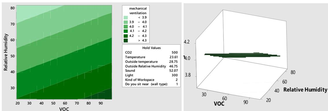
**Figure 7.** Relationship between relative humidity, VOC and indoor air comfort.
