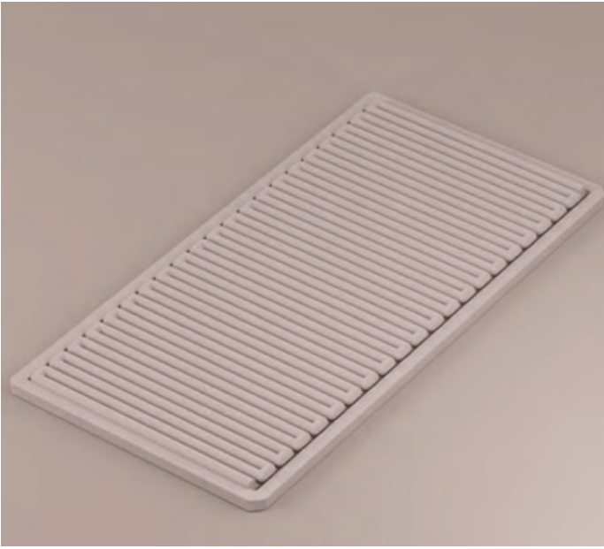
(a) Simulation of the deposition Simulation of the deposition of the 1st layer to create a 3D printed block using recycled aggregates. The type of pattern developed from the toolpath will help to reduce the amount of material hence reduce the CO 2 emissions.
